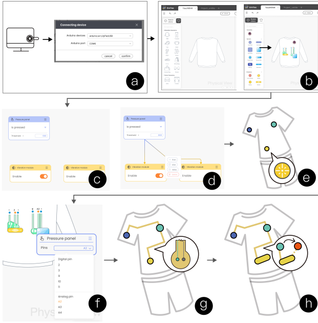
Figure 12: Prototyping workflow. a) Connect the control board, b) Simulate the design, c) Assign the functions, d) Edit the interactions, e) Place components and connectors, f) Set wiring pins, g) Connect the circuit, h) Test and iterate.
