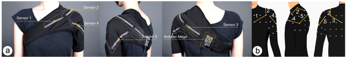
Figure 1: Overview of the wearable system. (a) A customized shoulder wrap equipping with five textile sensors, (b) The illustration of sensor placement. Five textile sensors were placed around the anterior and posterior fascicles of the deltoid, trapezius, pectoralis externus, and scapularis raisers.
