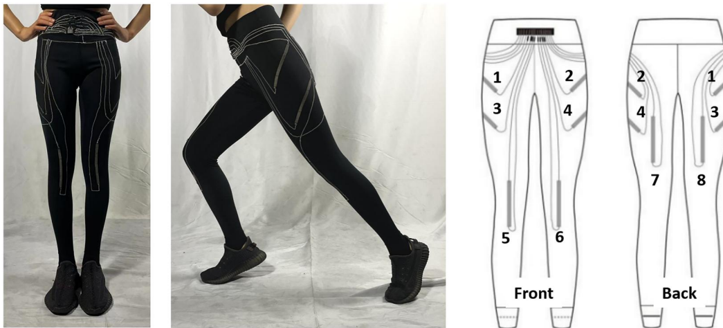
Figure 14. The layout of the 8 sensors on the smart leggings with front and back views.
